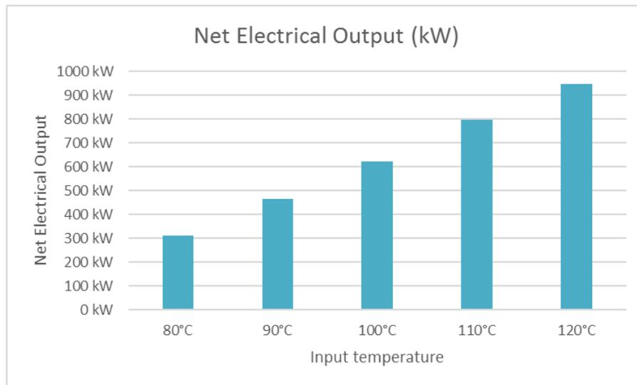
**Figure 4: Climeon Heat Power System performance from a resource with a flow of 30 liters per second at varying input temperature.**
