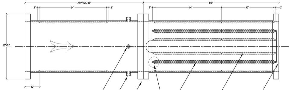
**Figure 1.** Drawing of 42 Inch Diameter Silencer Showing Locations of Resonant Acoustic Elements (Dashed Lines). Dimensions are in inches. Flow is left to right.
