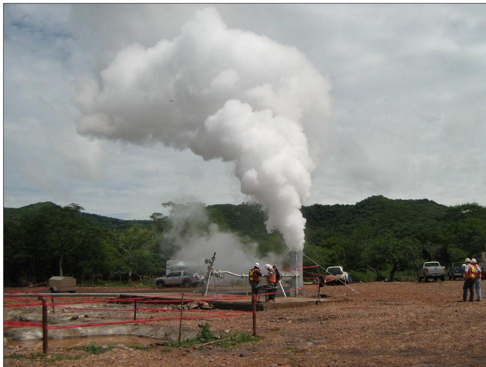
Figure 1. Discharge testing slimhole well MG-04, Mita Geothermal Field, Guatemala.
