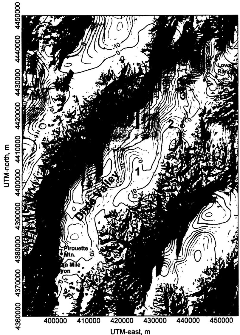
**Figure 1.** Residual Bouguer gravity anomaly map of the Dixie Valley area. Geothermal sites mentioned in the text are located and named.
