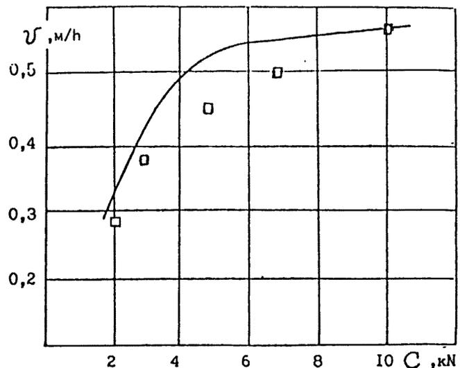
Figure 1. Experimental values and theoretical curve of dependence of rate of drilling by melting on axial load ( $\varnothing$  50 mm, H=75 mm) at active power of penetrator  $N_a = 5$  kW when applied to basalt.
